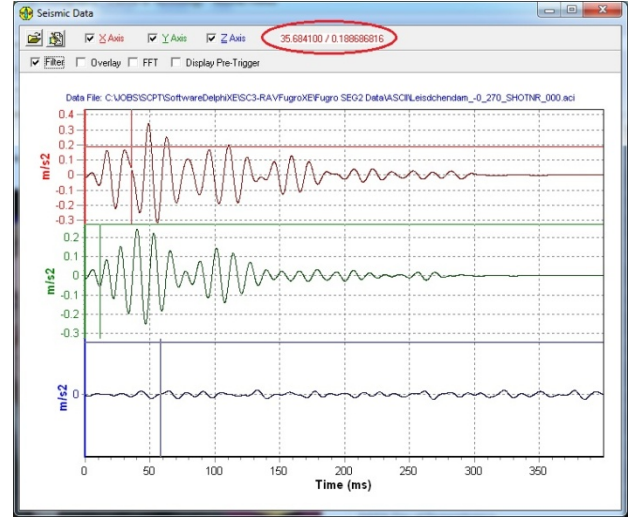
Figure 11: Utilities->View Seismic Data display with the Amplitude and Time default settings (Precision, Digits and Increment) set at 9, 9, 0.00001 and 6, 6, 0.00001, respectively
